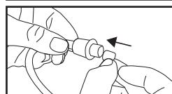
3. Insert a single-use filter into the end of the tube.
