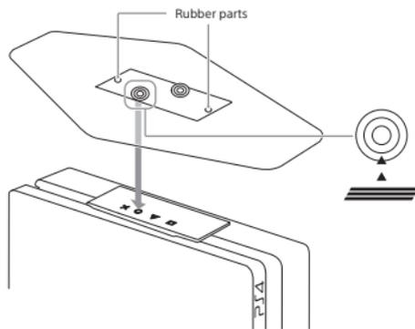
**4 Use a coin or similar flat object to tighten the mounting screw.**
